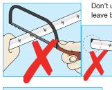
Don't use hacksaws to cut the pipe or leave burrs on the end of the pipe.
